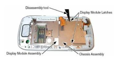
• Use the disassembly tool to release the display module assembly latches located under the chassis assembly.
