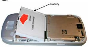
Press the battery cover latch on the bottom of the phone, and lift the battery cover up from the phone and lift it off.
