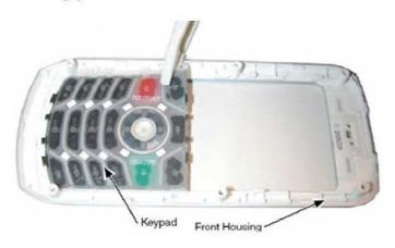
Lift the keypad up from one corner as Shown, and remove it from the front housing. 6.
