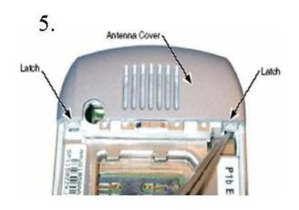
Use the metal tweezers to release the antenna cover latches.
