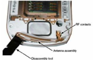
Use the disassembly tool to lift the side of the antenna out of the phone.
